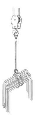
Fig.13 Choker hitch double wrapped
