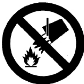
Do not extinguish with water
