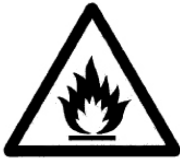
Flammable material or high temperature
