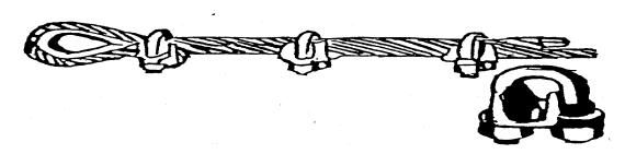
**NOTE:** There is only one correct method of installing wire rope clips. They should be attached to rope ends as shown in the photograph above. The base of each clip should bear against the live, or long rope end, and the U-bolt should bear against the dead or short rope end.
