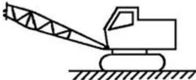
Self-propelling crawler track mounted crane
